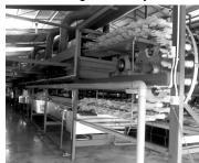
The glove chlorination system is used to produce powder-free rubber gloves. It involves the dipping or washing of rubber gloves in process tanks which contain diluted chlorine solution to reduce friction on the surface of the gloves, thus eases the donning of gloves without using powder.
